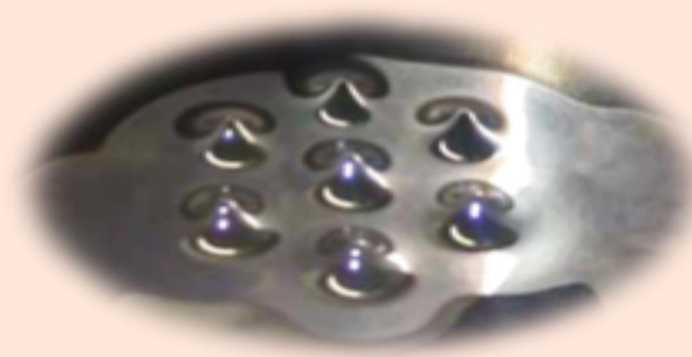
Localised hexagon on the surface of a ferrofluid [LGR+15]
